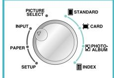
Select the method for input of image data, either by printing directly from a card or printing from a PC.
